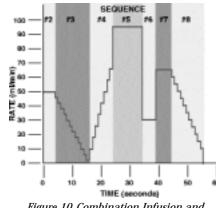
Here is an example of a more complex profile program. Each 'run' of the infusion has been determined to pump 43.155 ml. The first sequence refills the syringe with the volume to be infused then the infusion profile is started, after which the syringe is refilled and the infusion is repeated until the pump is stopped.
