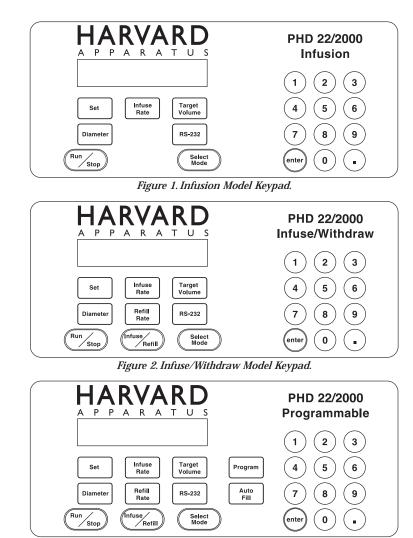
Figure 3. Programmable Model Keypad.
