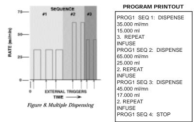
Here, a series of dispenses are programmed. Each dispense is started by a trigger, such as pressing the RUN/STOP key or pressing an attached foot switch. Seven dispenses are programmed: three of 15 ml at 35 ml/mn, two of 25 ml at 65 ml/mn, and two of 17 ml at 45 ml/mn. The pump's display will show 'TRIGGER' when it is waiting for a run trigger and < or > will not be displayed.
