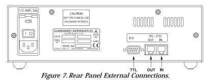
External devices that can be attached to the PHD 2000 are categorized into either RS-232 devices or TTL devices. Pump Chains, Scales and Printers are RS-232 devices, all other devices are TTL devices. See the Appendix F for specification details on attaching RS-232 devices and Appendix E for TTL.
