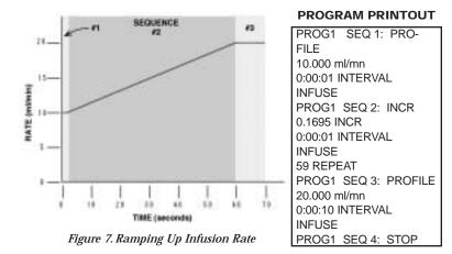
In this example, the pump will ramp up from 10 ml/mm to 20 ml/mn over 60 seconds, then continue to run at 20 ml/min for another 10 seconds. This is a Strategy 2 Program requiring four sequences:
